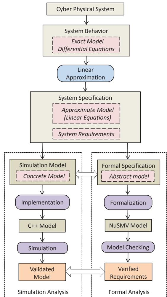
Figure 1 Proposed CPS System Analysis Methodology
